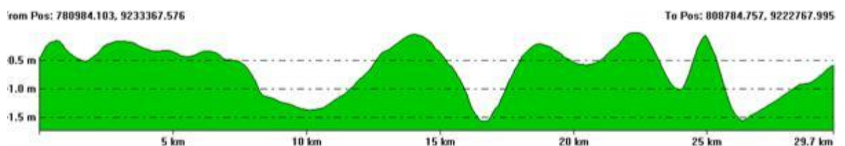
Figure 2.7: Land subsidence along transect a (ADB project, Annex F, figure 19)
