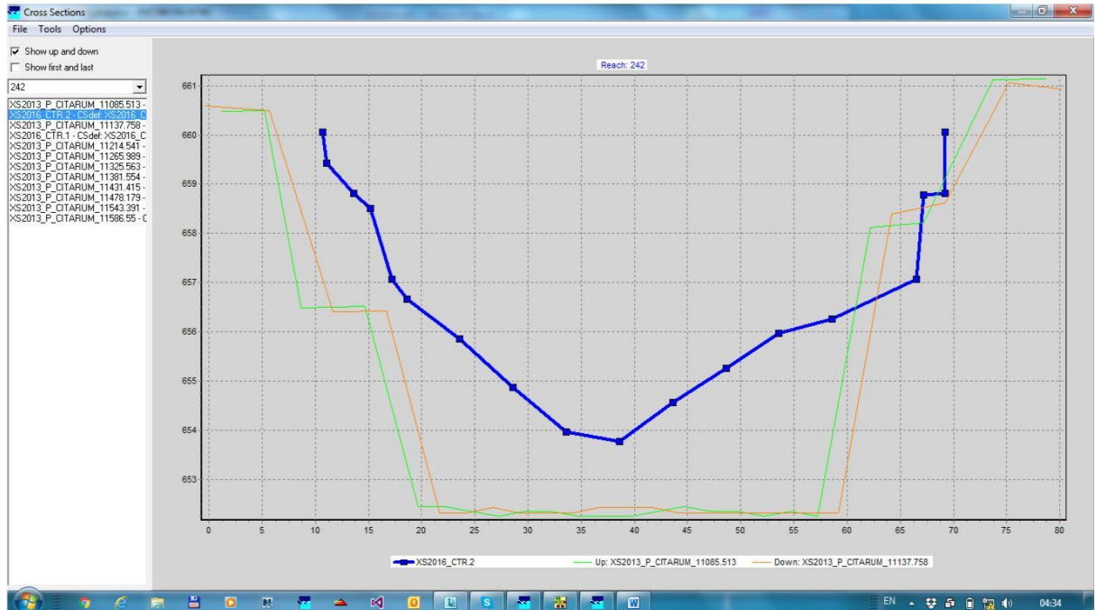
Figure 2.10: Cross-sections from 2013 and 2016 near Dayeuhkolot, downstream Cisangkuy confluence (dark blue = 2016 cross-section, green and orange are the upstream and downstream 2013 cross-sections)
